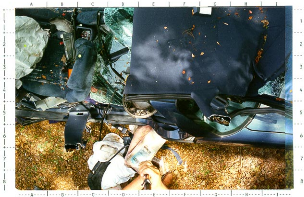
# 41 -- Overhead left center view of interior surface of 1991 Chevrolet Corsica's peeled-back roof; NOTE: no visible contact evidence
